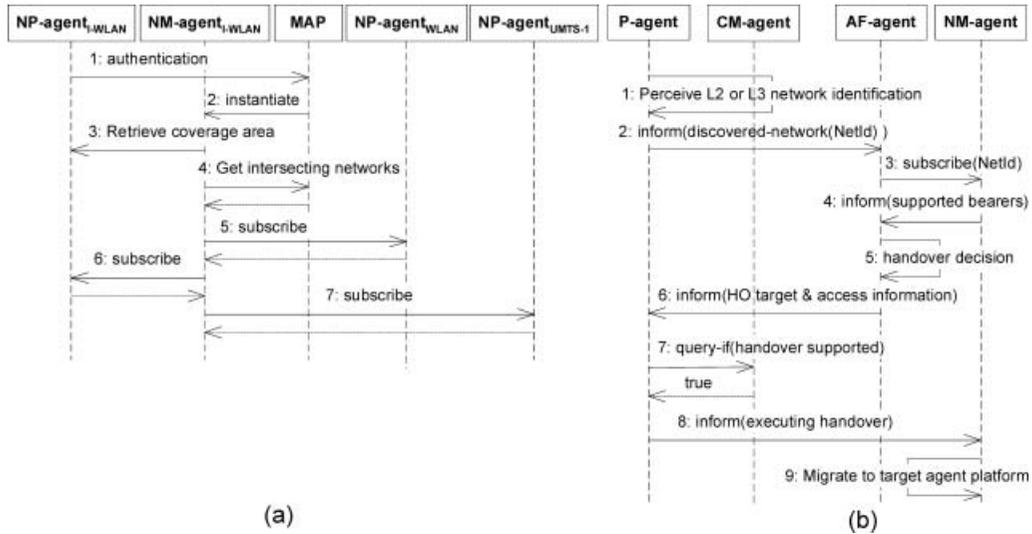
Fig. 3. (a) Bootstrapping of network provider's platform, (b) handover initiation and decision.
