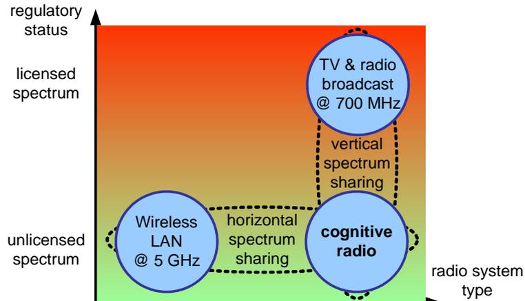
**Figure 6:** Cognitive radios share spectrum with different radio systems. Depending on regulatory status, vertical or horizontal spectrum sharing is done.
