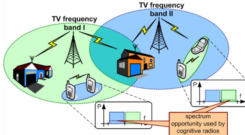
**Figure 7:** Cognitive radios operating in frequency bands of TV and radio broadcasts. At different locations the cognitive radios identify different frequencies as unused and regard them as spectrum opportunities. This example of vertical spectrum sharing is the basis for IEEE 802.22.
