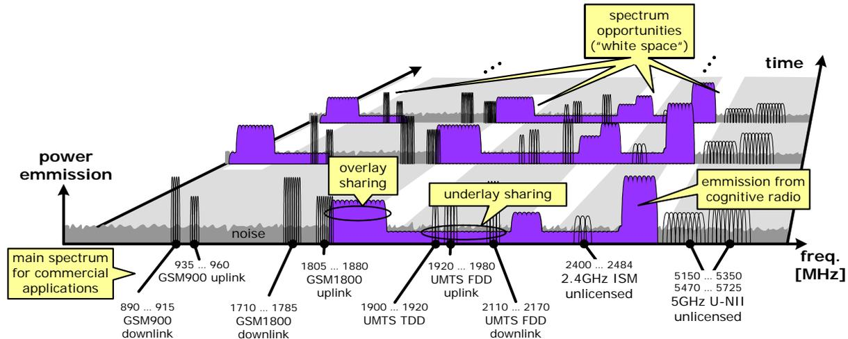
Figure 4: Underlay and overlay spectrum sharing of a frequency agile cognitive radio using spectrum on an opportunistic basis [17].
