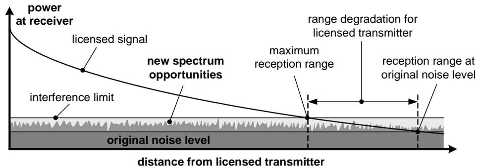
**Figure 5:** Underlay spectrum sharing corresponding to the Interference Temperature Concept of the FCC [16].
