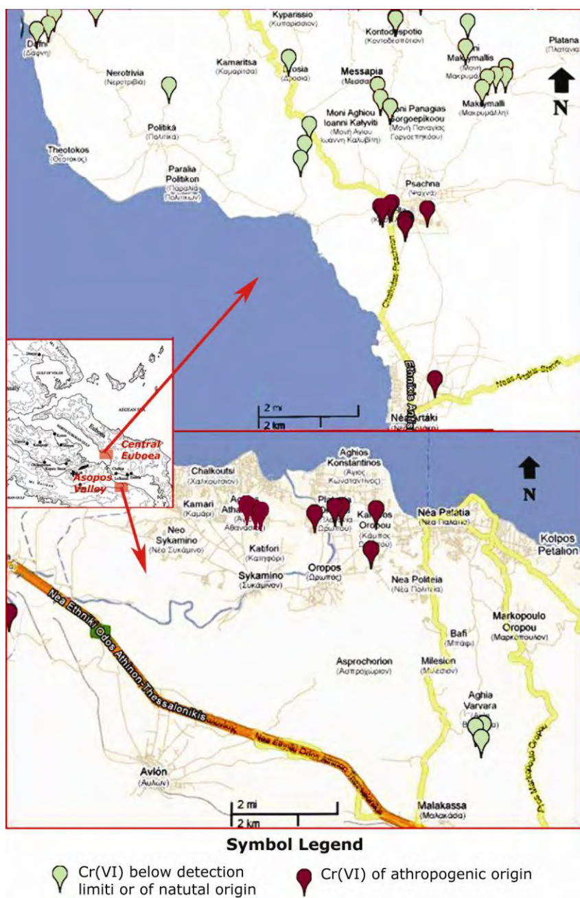
Fig. 4. Map presenting the suggested origin of Cr(VI) in the aquifers at Eastern Sterea Hellas. Lower: Asopos Valley, Upper Central Euboea (additional data from Vasilatos et al, 2008, and Megremi, 2010) .
